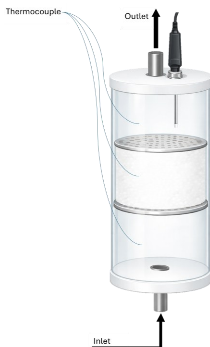
Figure 6. Schematic picture of the packed-bed reactor with humidity probe and thermocouples.
