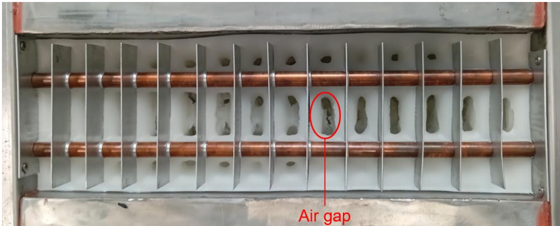
Figure 6. Air gaps visible in the PCM in heat exchanger A.
