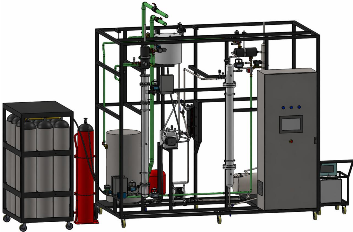
Figure 7. 3D design of the laboratory-scale PCC unit.
