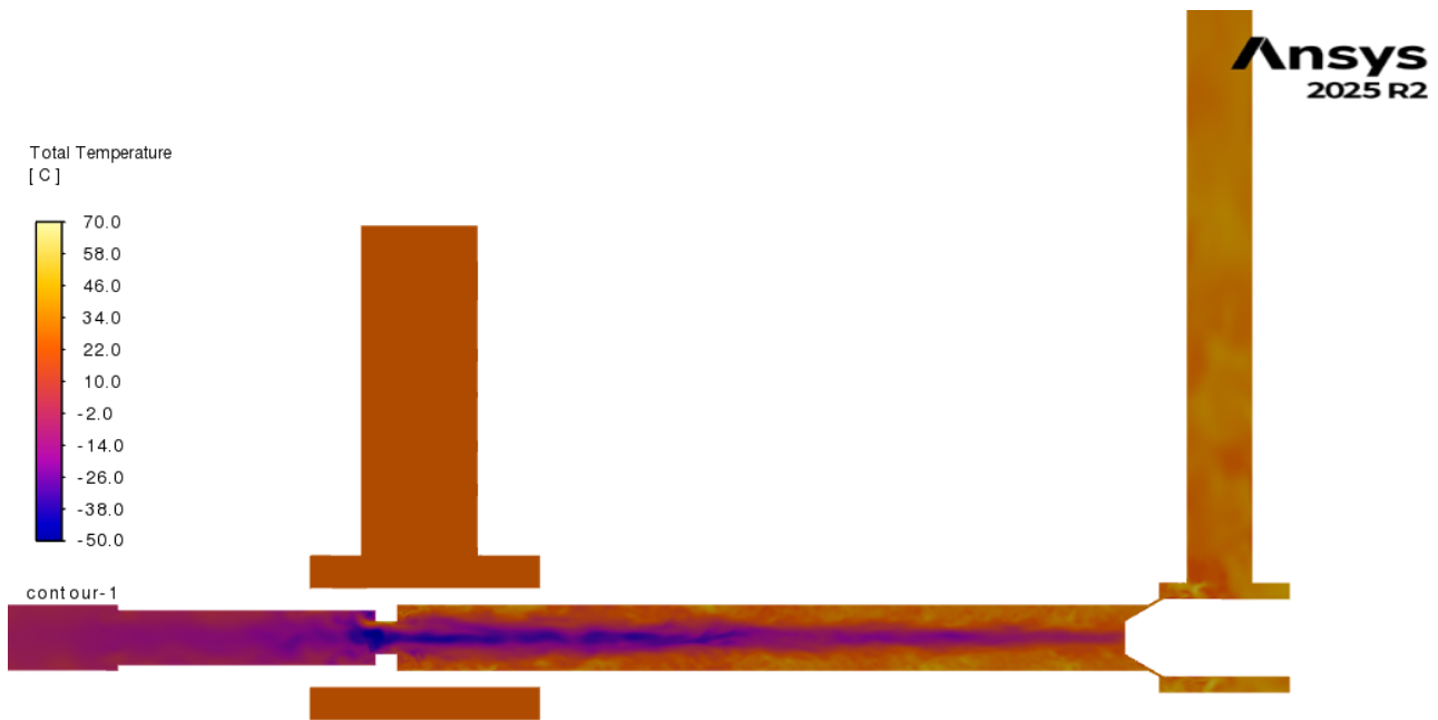
Figure 5: Counter of total temperature for the nitrogen simulation
