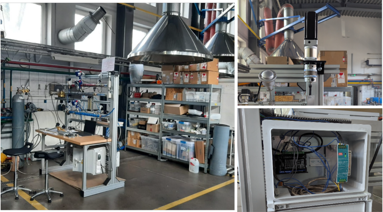
Figure 4: The RHVT test rig in the laboratories of SUT (left side) and regulation valve positioning system (right side).
