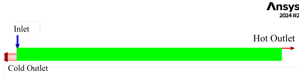
Figure 8: Schematc representation of the evaluated RHVT.
