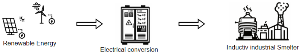
Figure 4: Schematic drawing of the CO 2 -neutral technology option smelting with an inductive smelter.
