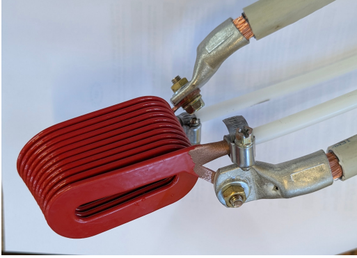
Figure 5: On the left, coil under test connected to power and coolant supply. On the right, example of temperature distribution along the coil during a test.
