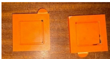
Figure 5. Mold used for custom gasket fabrication.
