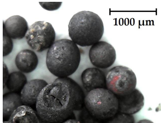
Figure 3. CuO/Al 2 O 3 oxygen carrier particles used in the study.
