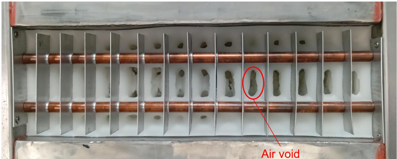
Figure 11. Air voids in the PCM.
