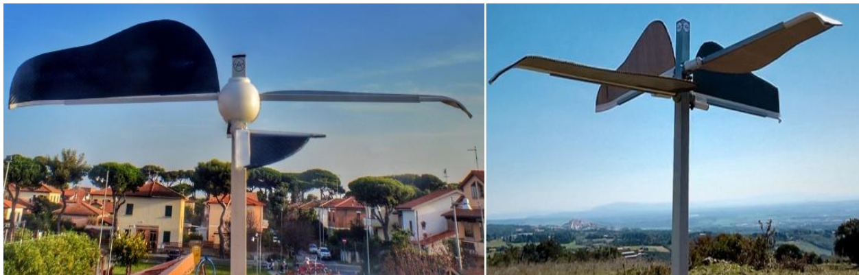
Figure 4: AIRON prototype with modular elements; comparison between system with and without semi-spheres.
