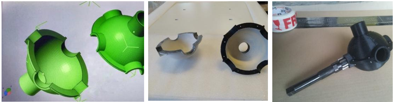
Figure 3: 3D-printed CAD hemispherical elements for coupling blades on the drive shaft.
