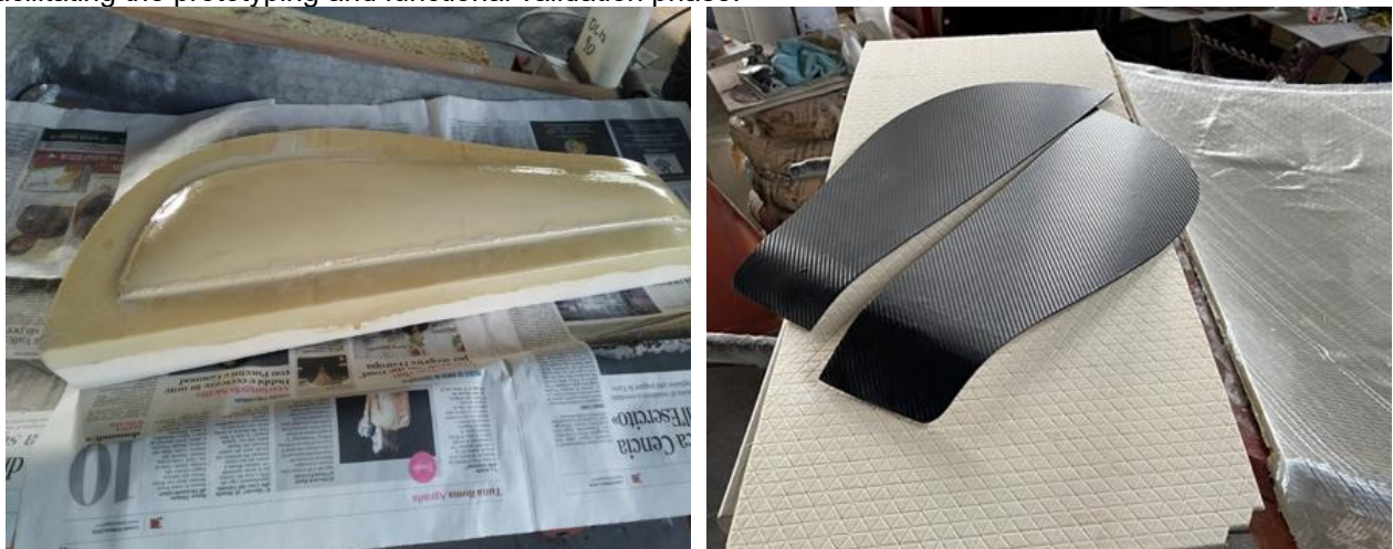
Figure 2: Blade mold and blades molded in carbon fiber.
